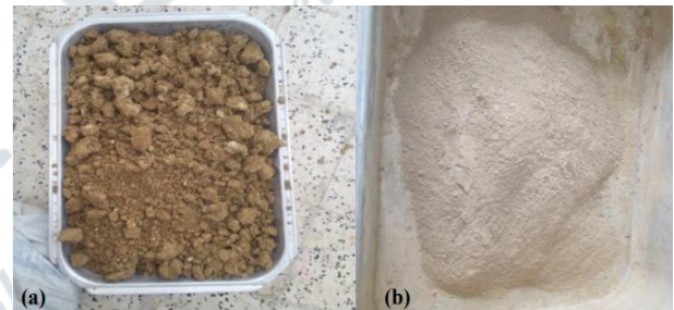
Fig.1. Clay used (a-Clay before crushing; b-Clay after crushing and sieving)
